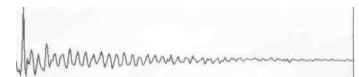
Fig.8 Apogee Centaur Minor, nearfield impulse response of rear panel's acoustic output (100ms time window, 1 kHz bandwidth)
